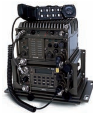
R&S®XV3088 (R&S®XV3088C) mobile system: The base unit is formed by the R&S®XV3088 transceiver, built- in into various frames together with the R&S®VV3088M (R&S®VV3088V) 25 W (50 W) power amplifier.
