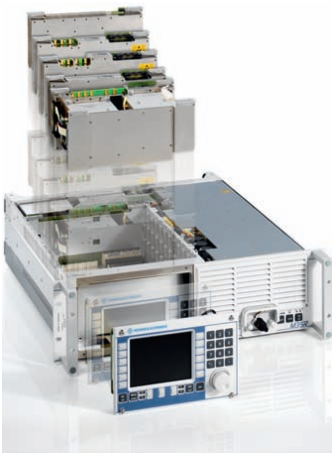
Modular design of the R&S®M3SR Series4400 radio family.
